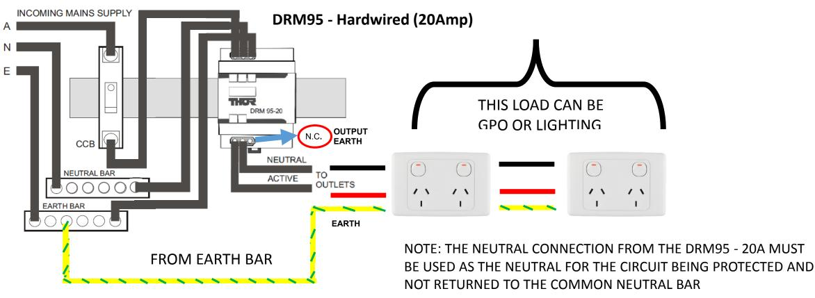
FOR A HIGHER LEVEL OF PROTECTION OF THE DRM95 IT IS RECOMMENDED THAT AN RCD DEVICE IS USED INSTEAD OF A STANDARD CCB. HOWEVER, IF YOU ARE USING AN RCD YOU CANNOT USE DRM95 INTERNAL EARTH YOU MUST USE THE MAIN EARTH BAR CONNECTION THEN THE INTERNAL CONNECTION ON DRM95 IS "N.C." NOT CONNECTED
